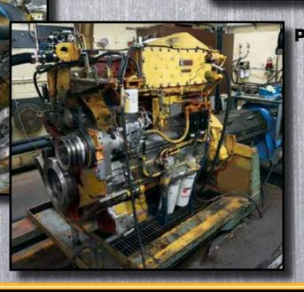
POWER TEST 2000hp 6000 lb. ft. torq. 4000 RPM max
